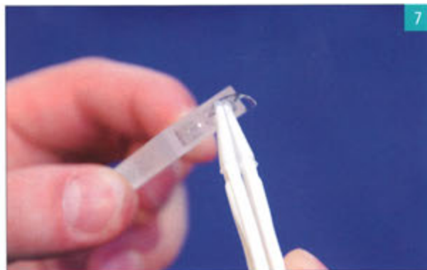
Fig. 7: Traditional plano wet cell for power mappers
