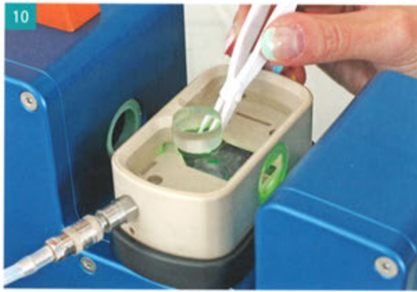
Fig. 10: Multi-functional open wet cell
